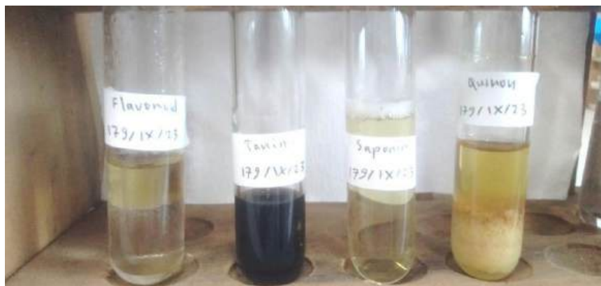
Figure 1. Positive flavonoids with yellow color change, positive tannins with blackish color change, positive saponins with foaming, and quinone is negative because there is a precipitate
